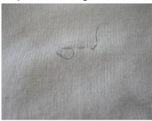
Black polypropylene (Bailing Twine) fibre in a fabric
