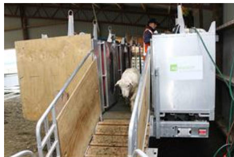
NZ ram breeders can now measure animals’ methane emissions, via Portable Accumulation Chambers.
