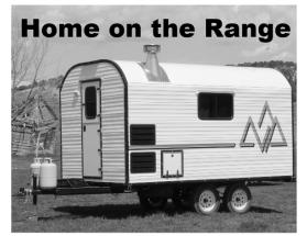
The Sanpitch Series camp is a staple in many sheep, cattle, and other livestock operations thru out the United States. This camp is generally built in the 18' to 22' range. It can be constructed on a variety of frames with running gear to match your needs (Tie-rod front end, fifth wheel, or tandem).
